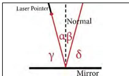
**Figure 1. Demonstration of the principle of light reflection**
